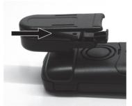
3. Secure the handset with the attachment clip to the belt. To do this, open the brackets by squeezing the free end and attach it to the belt.
