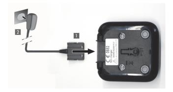
To disconnect the flat plug from the charger, press the release button and disconnect the flat plug.
